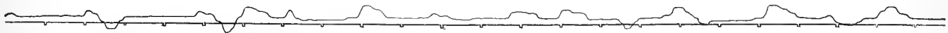
FIG. 6.—AUTOMATIC RECORD; HELM REQUIRED, SHIP NOT ROLLING (STRAIGHT LINE INDICATES RUDDER CENTER WITH ONE-MINUTE INTERVALS AS JCGS.)
